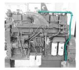
Fuel/Water Separator - Drain the water from the separator until see clean fuel
